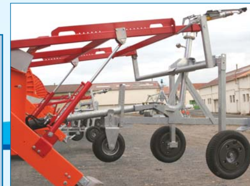
Hydraulic lifting 2000 series with separate drive
