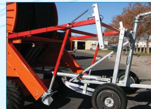
Hydraulic lifting connected to the lifting of the stabilizers (Premium type)
