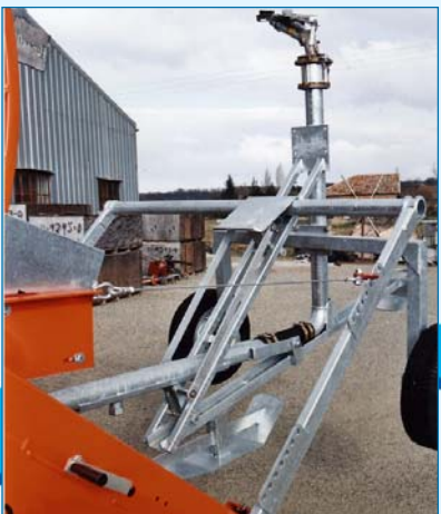
Automatic trolley lifting preventing crop-washing damages
